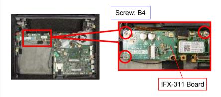
Remove the three screws, and then the IFX-311 Board.
