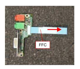
Disconnect the FFC. \*Pull it off in the arrow direction.
