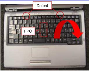
Disengage the two detents with a bamboo spatula, and turn the Keyboard toward the front.
