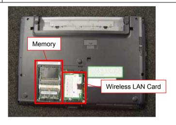
The Memory and the Wireless LAN Card are located under the Cover in section A.
