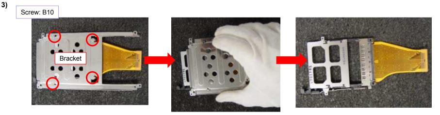
Remove the four screws, and then the Bracket.
