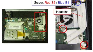
Remove the three screws, and then the Heatsink.
