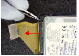
Disconnect the Connector portion little by little with a tweezers. \*Be careful not to bend the pins.
