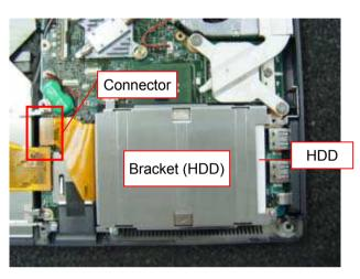
Disconnect the Connector, and remove the HDD.
