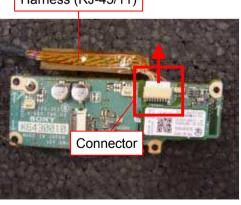
Disconnect the Connector in the arrow direction, and remove the Harness (RJ-45/11).
