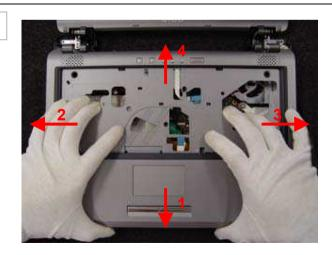
Raising the Palmrest while sliding it a little in the arrow direction in the order of 1, 2, 3, 4, disengage the detents.
