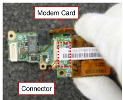
Remove the Modem Card. \*The Connector is located on the back.
