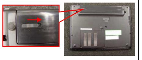
Slide the Battery Lock (L) to the UNLOCK side.
