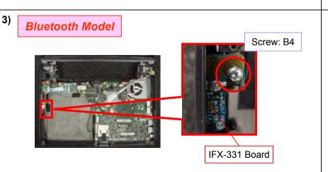
Remove the one screw, and then the IFX-331 Board.
