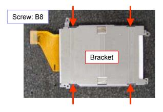
Remove the four screws, and then the Bracket (HDD).
