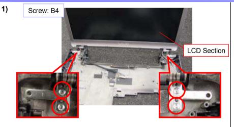
Remove the four screws, and then the LCD Section upward.
