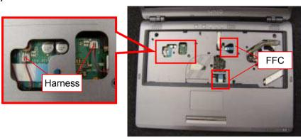
Disconnect the Harness (two places) and the FFC (two places). \*Pull off the Harness and the FFC upward.
