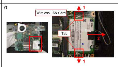
Turn over the Mother Board, open the tabs outward (arrow 1), and pull off the Wireless LAN Card diagonally upward (arrow 2).
