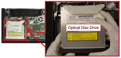
Remove the Optical Disc Drive.
