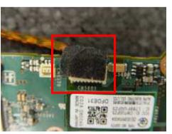
Turn over the IFX-311 Board, and peel off the Sheet.
