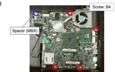
Remove the four screws and the Spacer (MBX) (one location). \*Remove the Spacer (MBX) using the 4 mm socket wrench.
