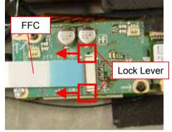
Slide the both ends of the lock lever in the arrow direction to unlock, and disconnect the FFC.
