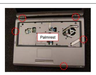
Disengaging the five detents, remove the Palmrest. \*The detents are engaged toward the outside.
