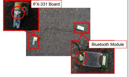
Disconnect the Coaxial Cable from the IFX-331 Board and the Bluetooth Module respectively.
