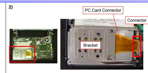
Disconnect the Connector, and remove the PC Card Connector.
