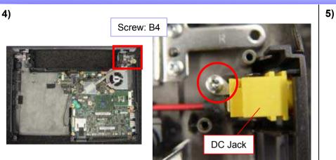
Remove the one screw, and then the DC Jack.
