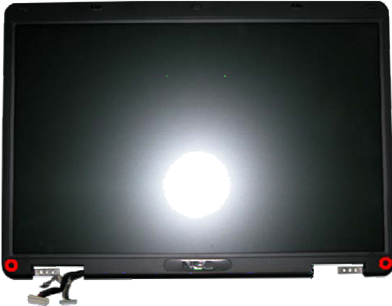
Fig. 25 Screws on the LCD Module
