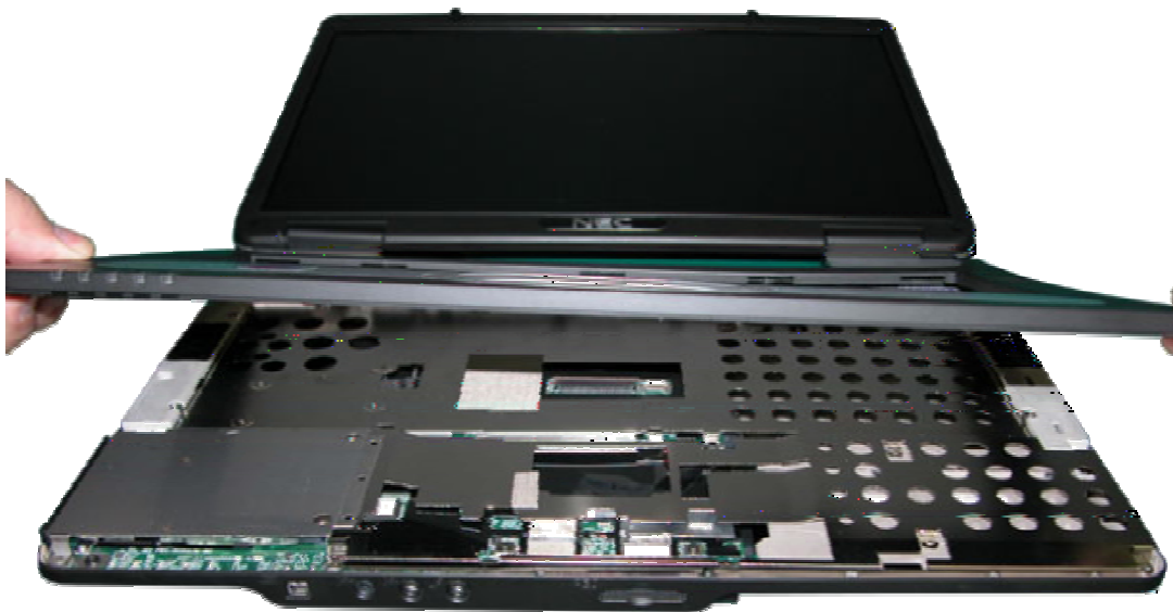
Fig. 20 Removing the Top Cover
