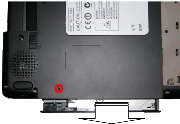
Fig. 6 Removing the optical drive
