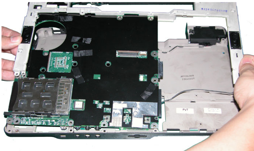
Fig. 32 Lifting up Main board
