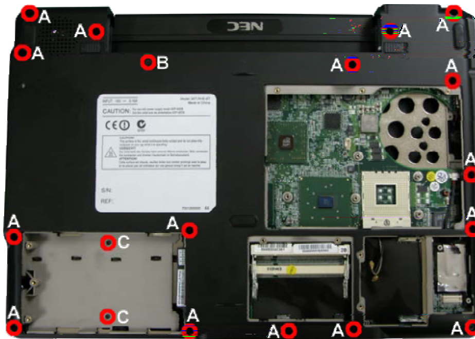
Fig. 18 Removing the top cover screws
