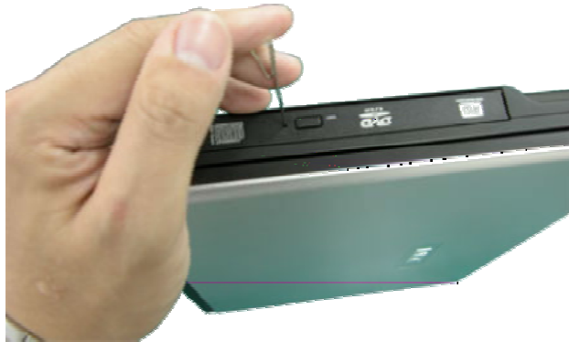
Fig. 5 Ejecting ODD tray
