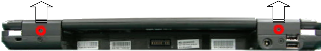
Fig. 21 Releasing LCD hinge cover
