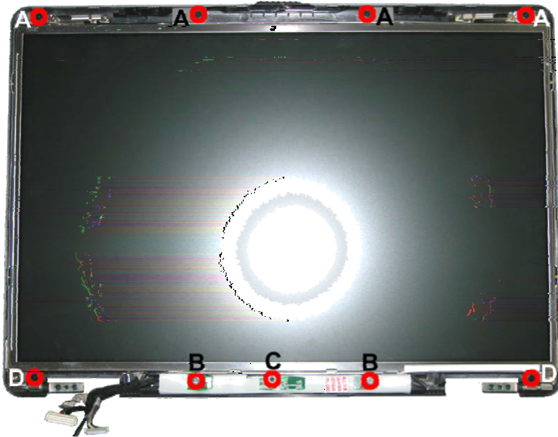
Fig. 27 Removing the LCD panel screws
