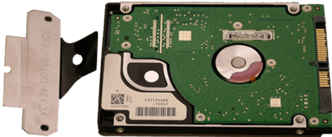
Fig. 4 The HDD and its bracket.
