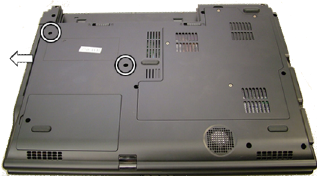
Fig. 5 The optical drive screws.
