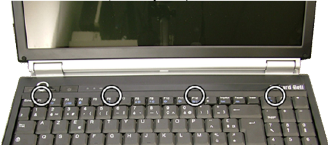
Fig. 16 The keyboard clips.
