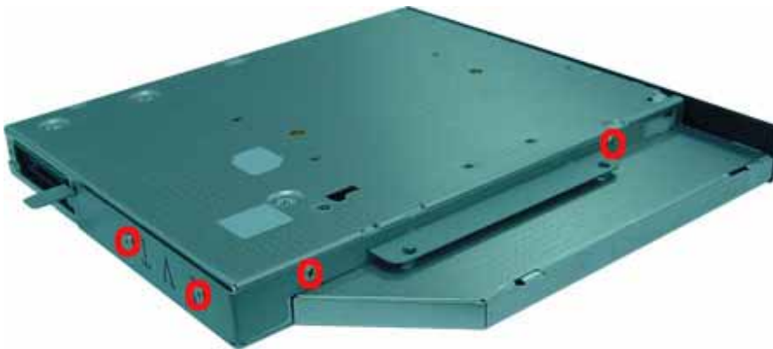
Fig. 7 Removing the Optical Drive Bracket
