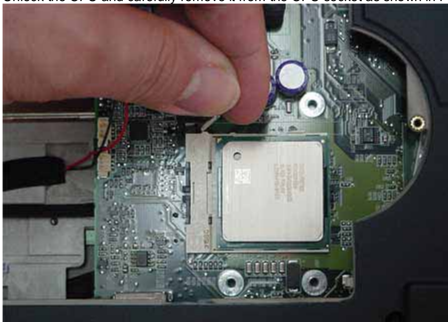
Fig. 31 Unlocking the CPU
