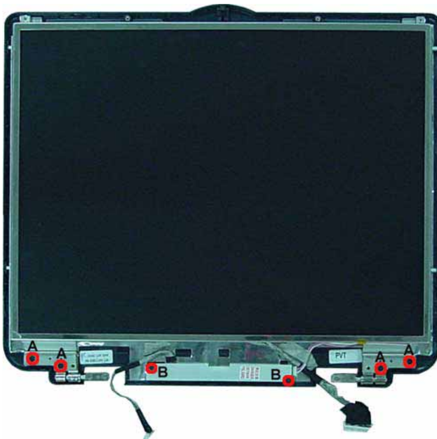
Fig. 19 Removing the LCD panel screws
