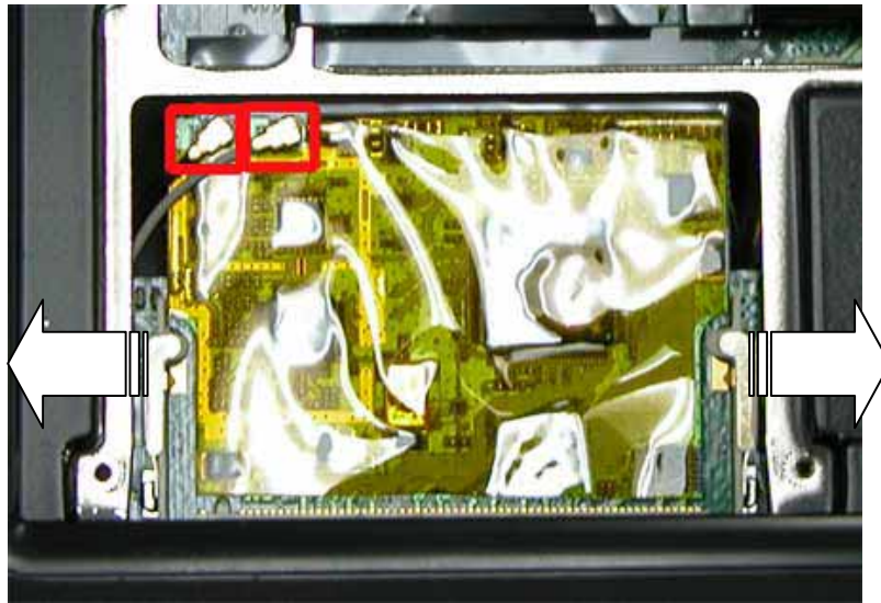
Fig. 41 Removing the WLAN Module
