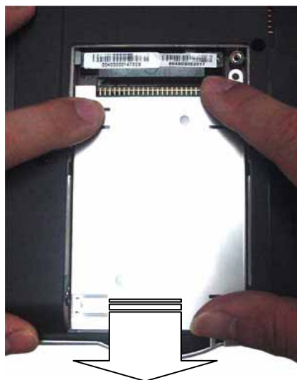
Fig. 3 Disconnecting the hard disk drive
