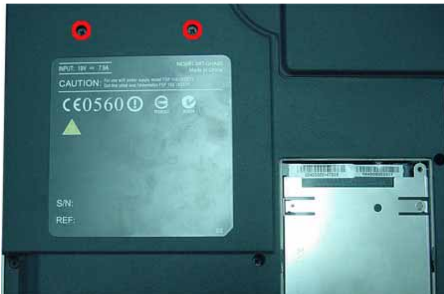
Fig. 5 Releasing the optical drive
