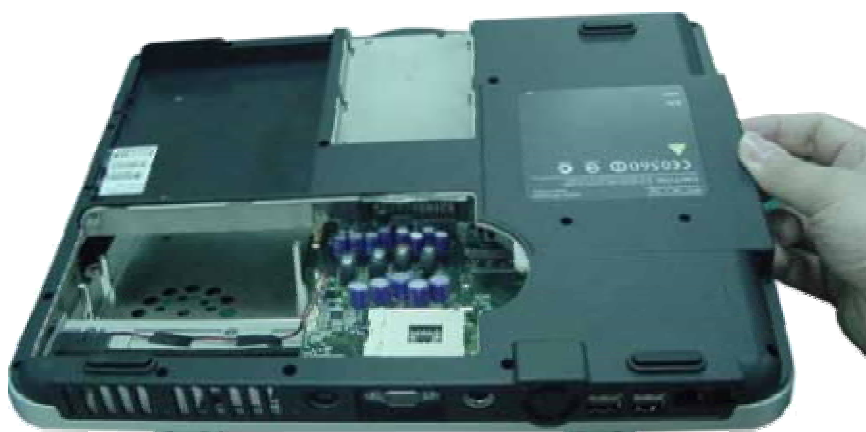
Fig. 36 Removing the Bottom Cover
