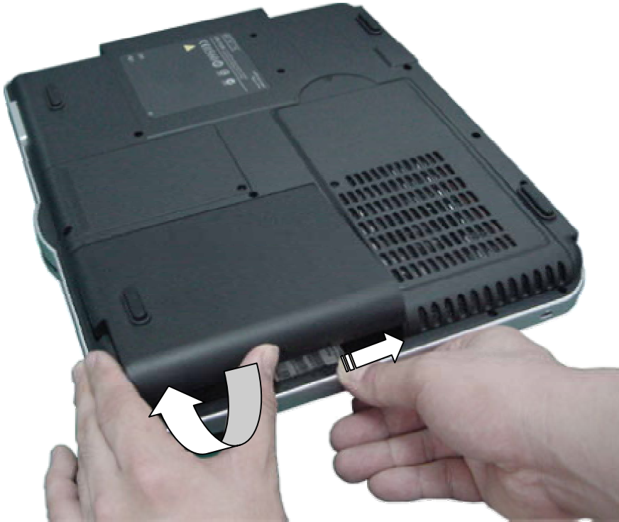
Fig. 1 Removing the battery
