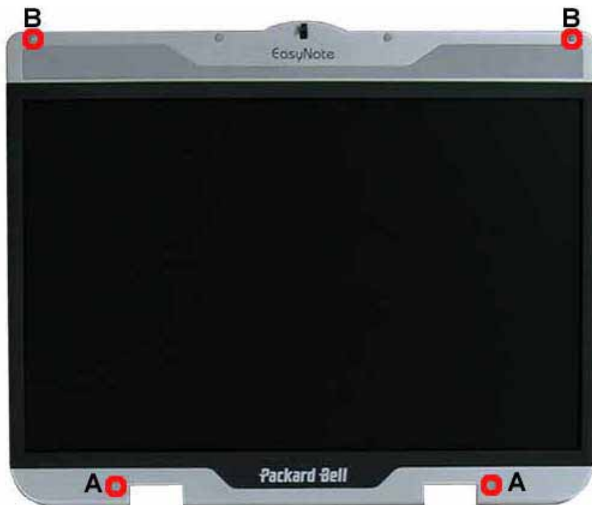
Fig. 23 Screws on the LCD Module
