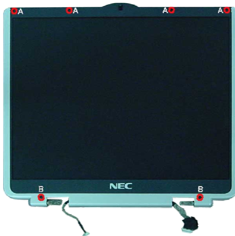
Fig. 17 Screws on the LCD Module
