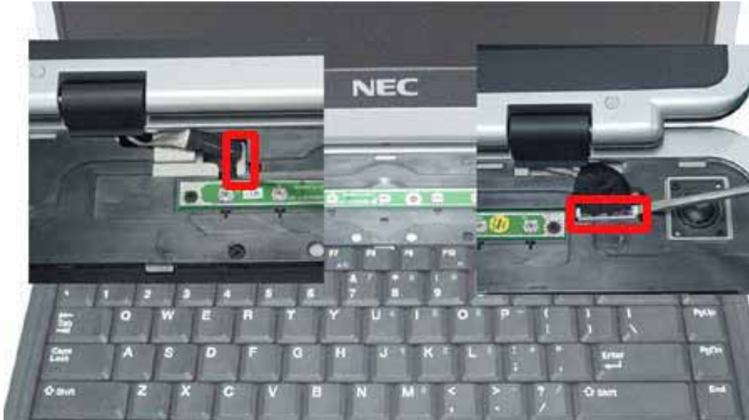
Fig. 13 Disconnecting LCD Connector
