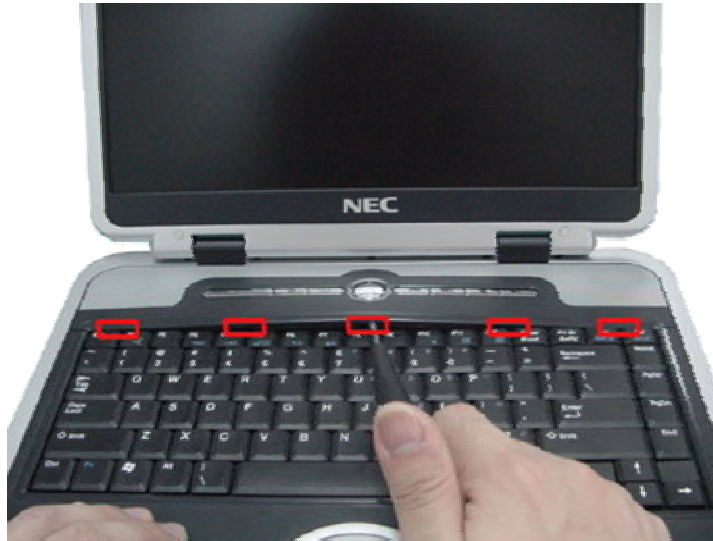
Fig. 8 Removing the Keyboard Cover
