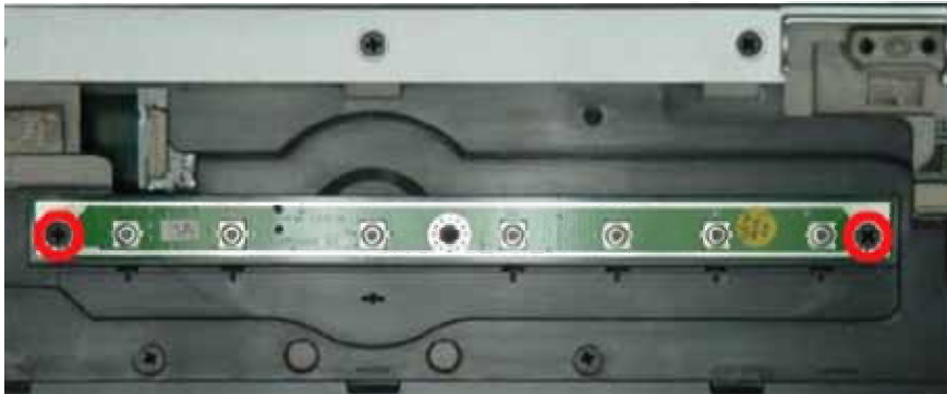
Fig. 32 Removing the Quick Key Board
