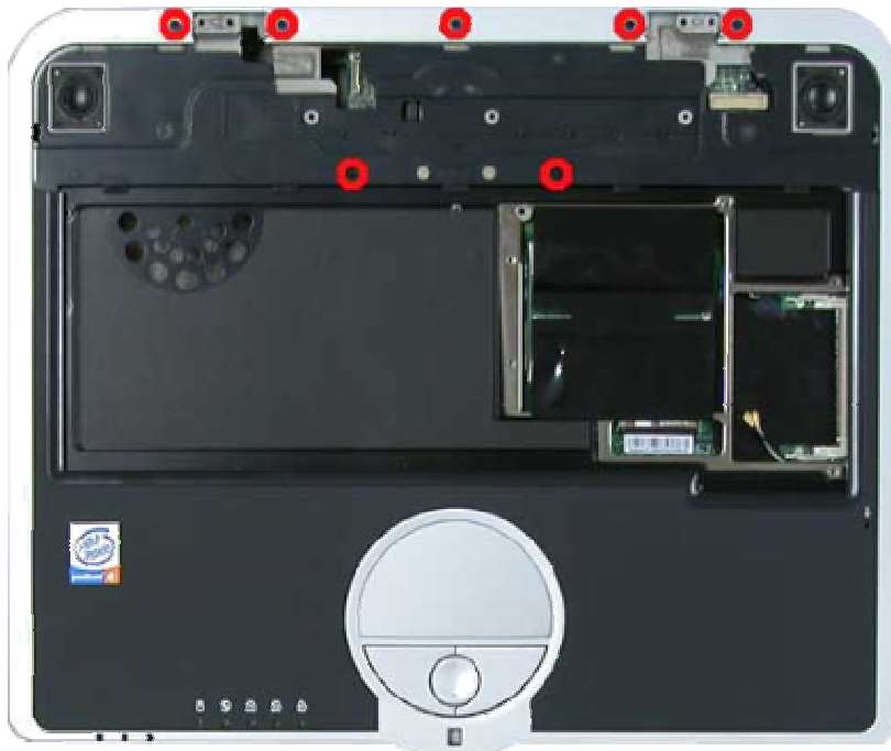
Fig. 33 Removing the top cover screws
