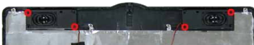
Fig. 28 Removing the Speakers
