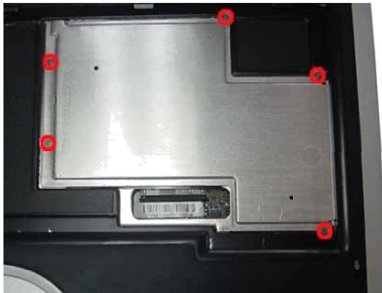
Fig. 11 Removing the screw retaining the memory module slot cover
