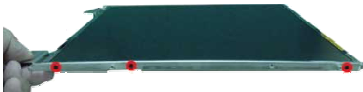
Fig. 27 Removing the LCD Panel hinges
