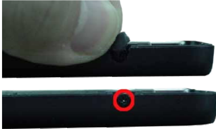
Fig. 20 Remove Side Rubber Cover
