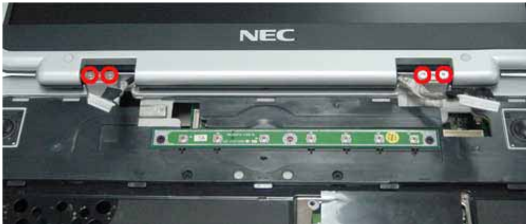
Fig. 15 Releasing the LCD Hinges
