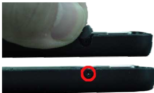
Fig. 26 Removing the Side Rubber Covers
