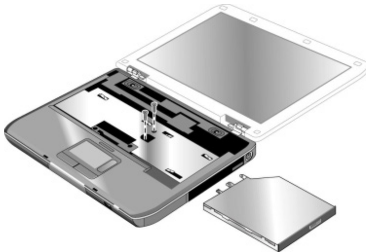
Figure 2-15. Removing the CD/DVD Drive
