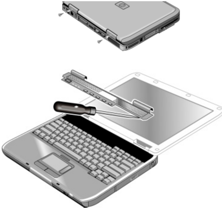
Figure 2-9. Removing the Keyboard Cover
