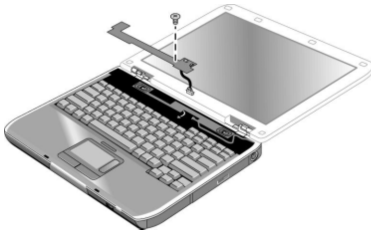
Figure 2-13. Removing the Switchboard PCA
