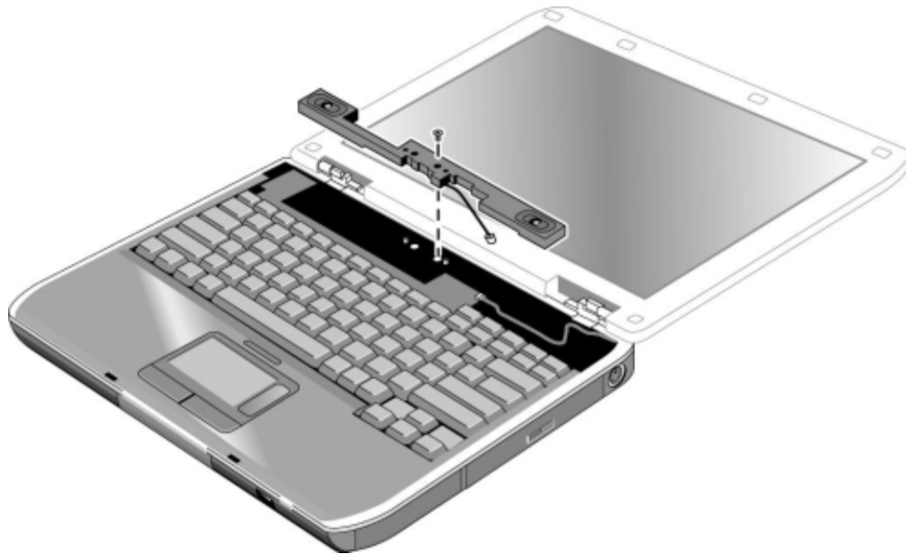
Figure 2-11. Removing the Speaker Assembly
