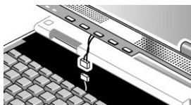
Figure 2-10. Disconnecting the Speaker Cable
