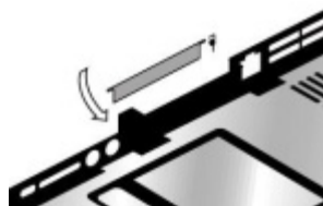
Figure 2-40. Removing a PCMCIA Door
