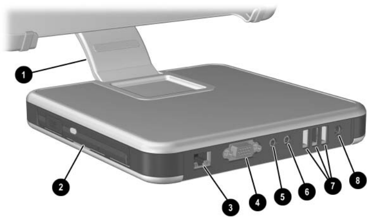
Docking Station Front and Left-Side Components
