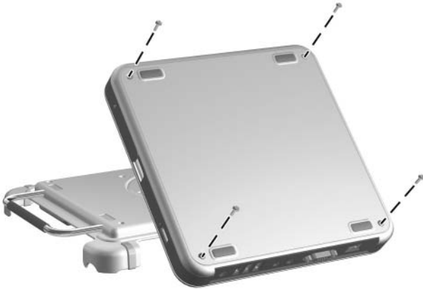
Removing the Top Case Screws
