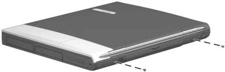
Figure C-13. Phillips M2.5 × 9.0 Screw Locations
