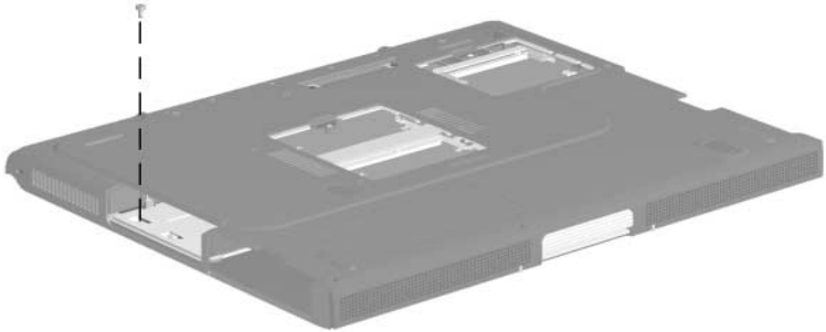
Figure C-8. Phillips M2.0 × 4.0 Screw Locations
