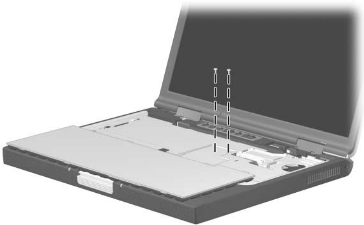
Figure C-7. Phillips M2.0 x 4.0 Screw Locations
