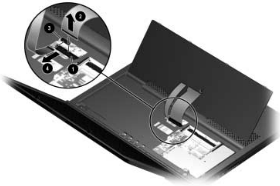
Figure 5-19. Disconnecting the Pointing Device and the Keyboard Cables
