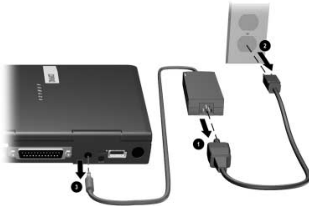
Figure 5-3. Disconnecting the Computer
