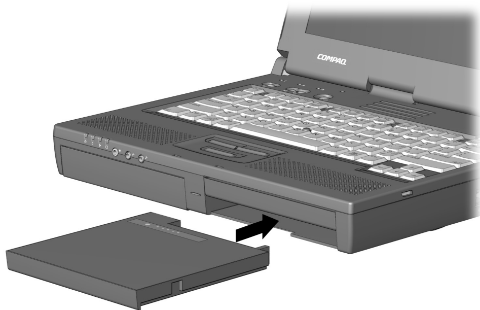
Figure 5-11. Inserting a MultiBay Battery Pack
