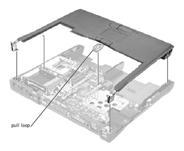
NOTICE: The reserve battery provides power to the computer's time RTC and NVRAM when the computer is turned off. Removing the palmrest disconnects the reserve battery and causes the computer to lose the date and time information as well as all user-specified parameters in NVRAM. If possible, make a copy of this information before you disconnect the reserve battery.
