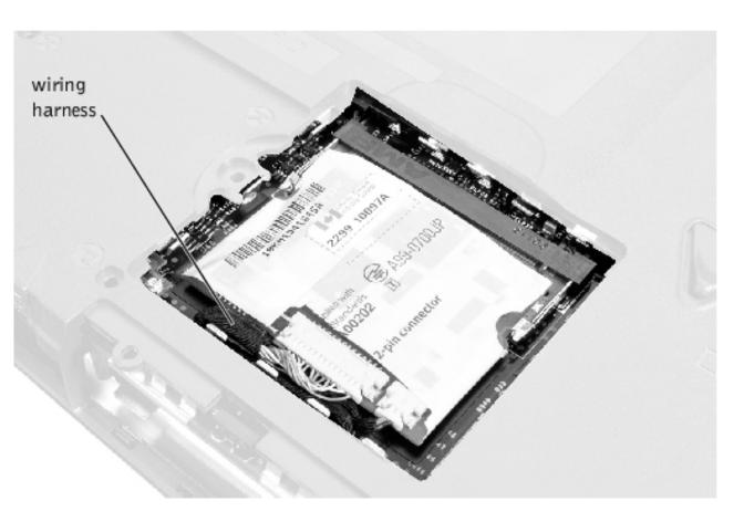
**Mini-PCI Wireless NIC Assembly Using Antenna Cable**
