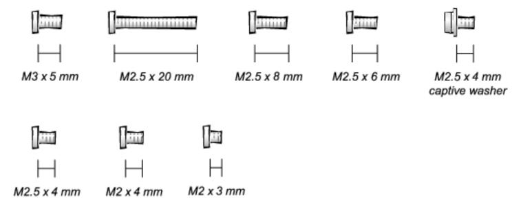
NOTICE: When reinstalling a screw, you must use a screw of the correct diameter and length. Make sure that the screw is properly aligned with its corresponding hole, and avoid overtightening.
