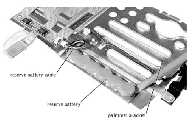
NOTICE: The reserve battery provides power to the computer's RTC and NVRAM when the computer is turned off. Removing the battery causes the computer to lose the date and time information as well as all user-specified parameters in NVRAM. If possible, make a copy of this information before you remove the reserve battery.
