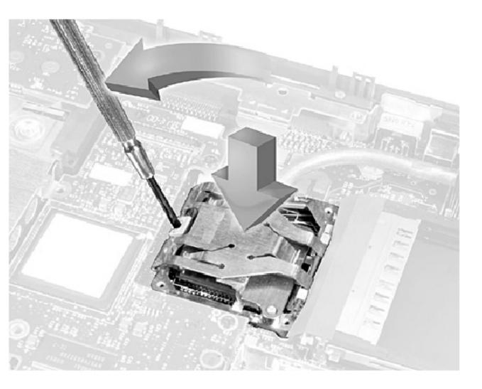
4. While pressing lightly down on the center of the retaining clip, insert a flat-blade screwdriver into the latch mechanism and pivot the top of the screwdriver away from
