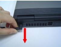
3. Turn the notebook over. Unlock and hold the latches, and remove the battery.
