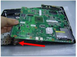
3. Remove 1 screw on the IO bracket.
