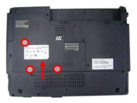
**Install battery module.**Put the battery module into its compartment.
