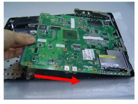
6. Secure 1 screw here and then connect the Bluetooth cables in the motherboard.
