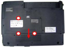
2. Pull two Latches and pop the module up to a 45° angles, and then pulling out the module in that angle.
