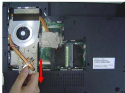
2. Turn the non-removable screw here 180 degrees counter-clockwise to loosen the CPU.
