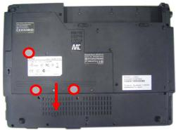
2. Remove 2 screws and Push the module out.
