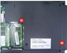
2. Put the CPU cover on and secure 3 screws (M2\*4L(K)) to fix it.
