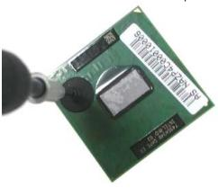
2. Install the CPU and use a single-slotted screwdriver to fix it.
