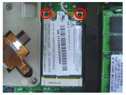
2. Connect the 2 antenna cables (black cable should be connected on main).
