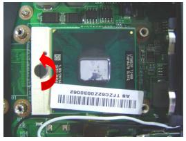
3. Squeeze the vacuum handling pump and use it to lift the CPU away.
