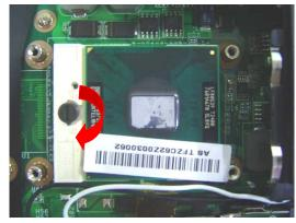
3. Install the CPU heat sink module gently and secure 7 screws upon the CPU module, then connect the fan cable.
