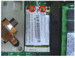
2. Remove 2 screws, then take the WLAN module away.
