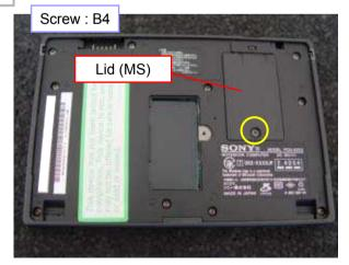
After removing the one screw, the Lid (MS) is removable.
