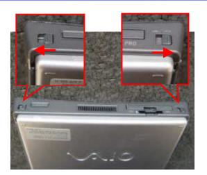
Slide the lever outward and release the lock.
