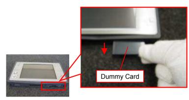
Pull out the Dummy Card in the direction of the arrow.
