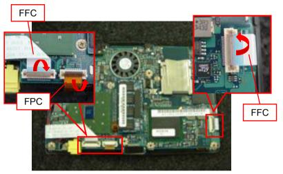
Raise the lock lever and remove the FFC (two places) and FPC (one place).
