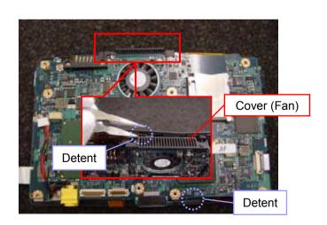
Disengage the detents (two places).
