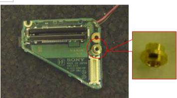
The Stand is installed under the Modem Card.
