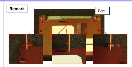
When the Keyboard can not be removed, insert the bamboo skewer from the back into the screw holes (three places) and release the keyboard.
