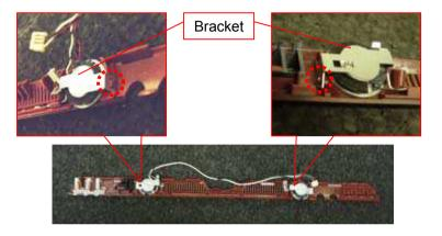
Remove the Bracket (two places) while disengaging the detent (each one place).
