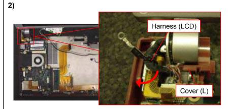
Pull out the Harness (LCD) from under the Cover (L).
