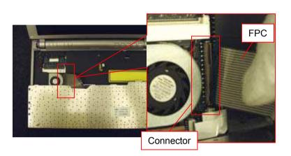
Disconnect the FPC. \*Raise the connector and release the lock.
