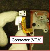
Remove the Connector (VGA).
