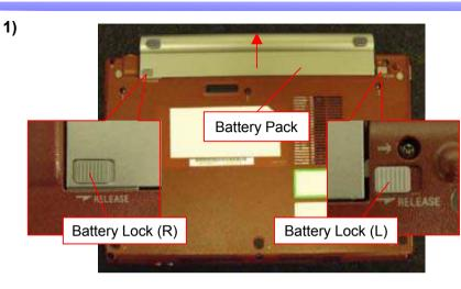
Remove the Battery Pack while moving the Battery Lock (L) and the Battery Lock (R) to the **RELEASE** side.
