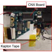
Peel off the Kapton Tape and remove the CNX Board. \*There is the Modem Card on the rear. 8)
