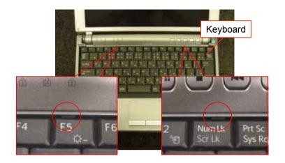
Disengage the detent (two places) and release the Keyboard. \*Push the detent with the bamboo spatula and disengage it.
