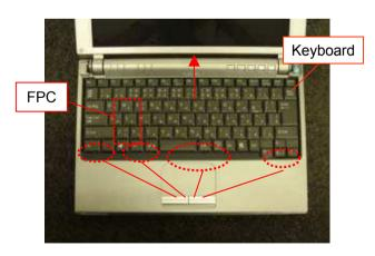
Slide the Keyboard in the direction of the arrow, disengage the detent (four places) and turn down the front side. \*The FPC is connected to the rear.
