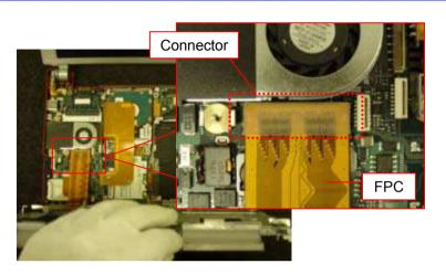
Disconnect the FPC. \*Disconnect the connector vertically.
