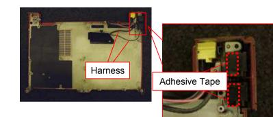
Remove the Harness (two places). \*The adhesive tapes are attached to the rear. 2)
