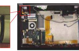
Remove the one screw. \* The screw secures the lug terminal.
