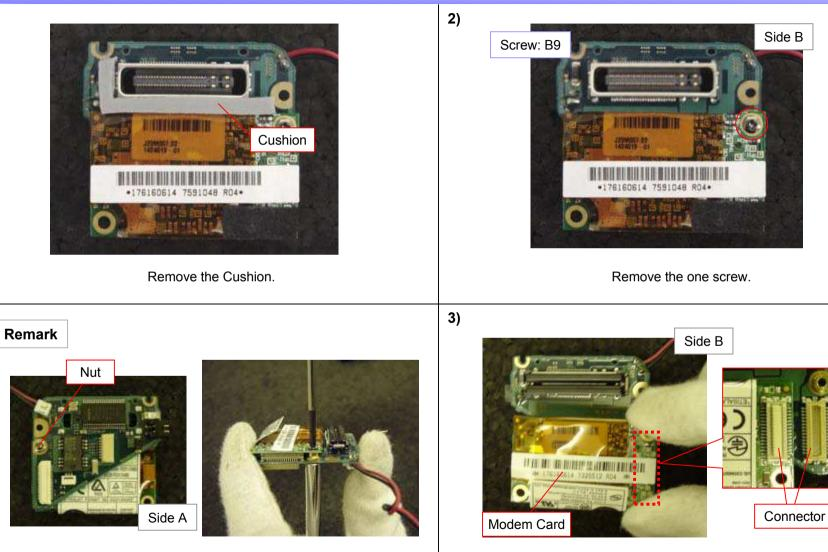
Remove the screw while securing the Nut of the side A with the 4 mm socket wrench.
