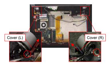
Remove the Cover (L) and the Cover (R) in the direction of the arrow while disengaging the detent (each one place).
