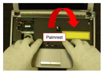
Pull the Palmrest toward the front, and raise the Palmrest to the front side while disengaging the detent (two places). \*The detent is engaged toward the outside.
