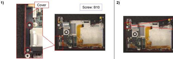
Remove the two screws and the Cover.
