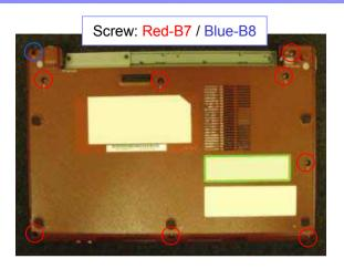
Remove the nine screws from the Bottom.
