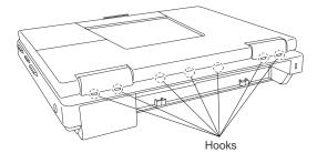
Release the seven Hooks fixing the rear side of the Center Cover.
