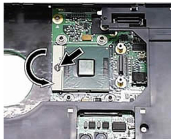
Fig. 14: Removing the CPU
