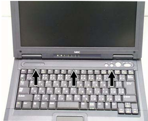
Fig. 7: Removing the keyboard cover
