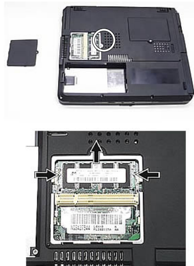
Fig. 2: Removing the memory module
