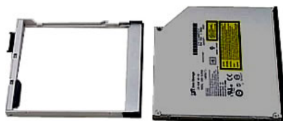
Fig. 56: Separating the optical drive from its frame
