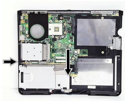
Fig. 39: Removing the main board
