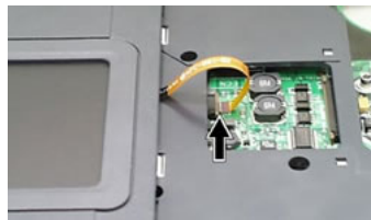
Fig. 22: Disconnecting the glide pad flat cable
