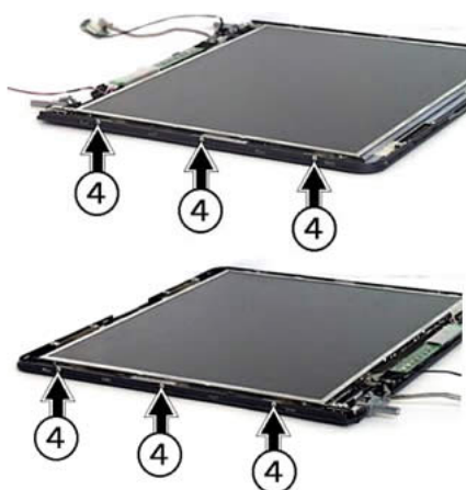
Fig. 48: Removing the screws retaining the LCD
