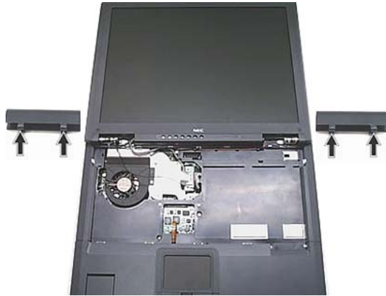
Fig. 15: Removing the plastic hinge covers
