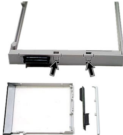
Fig. 57: Disassembling the plastic frame
