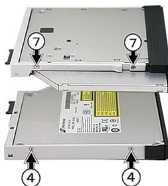
Fig. 55: Removing the screws retaining the frame of the optical drive
