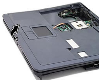
Fig. 24: Removing the glide pad assembly
