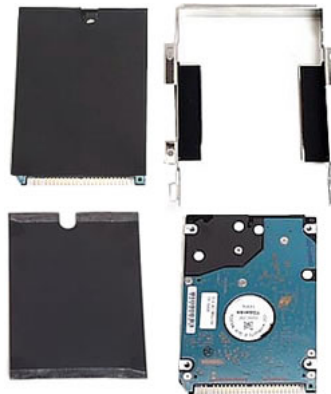
Fig. 29: Removing the hard disk drive
