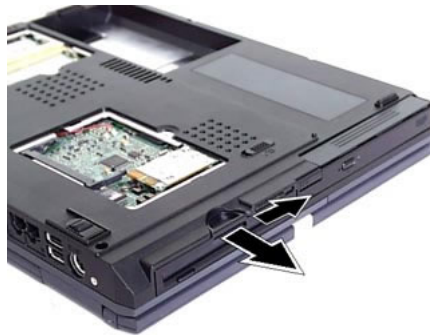
Fig. 6: Removing the Versa Bay IV optical drive
