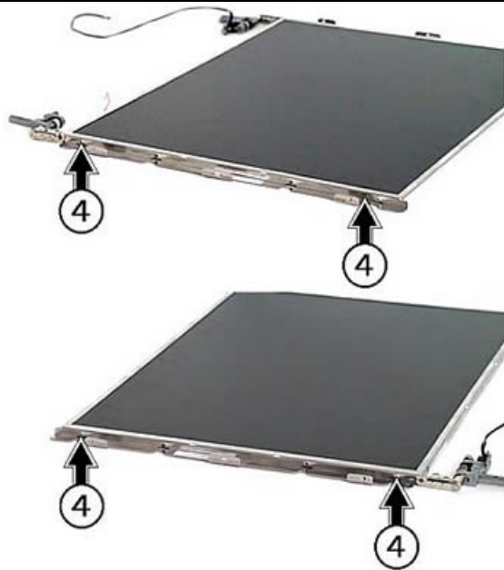
Fig. 52: Removing the LCD left and right hinges assembly
