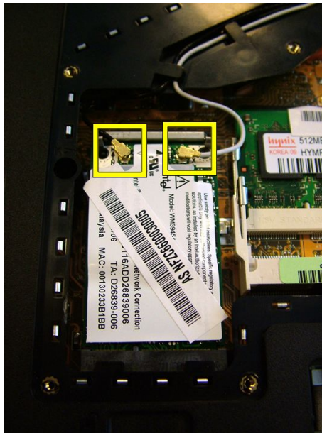
Fig. 5 Location of WLAN antenna cable connectors.
