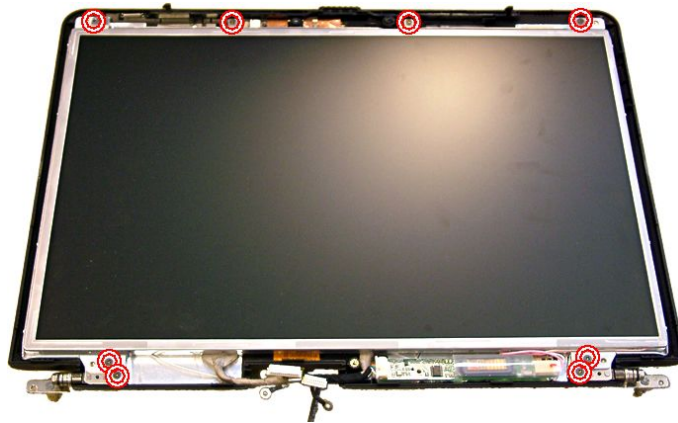
Fig. 28 Location of screws securing LCD module.
