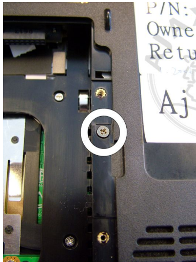
Fig. 4 Location of optical disk drive screw.
