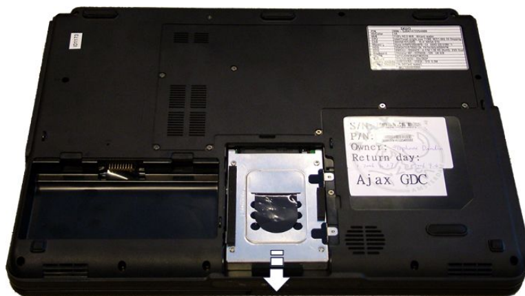
Fig. 2 Removing hard disk drive.
