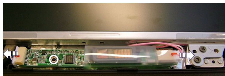
Fig. 27 Location of inverter board.
