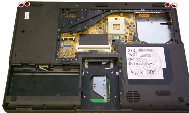
Fig. 12 Removing 4 bottom screws.
