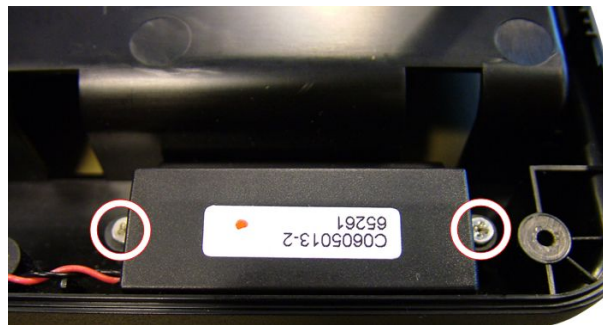
Fig. 23 Location of speaker assembly screws.
