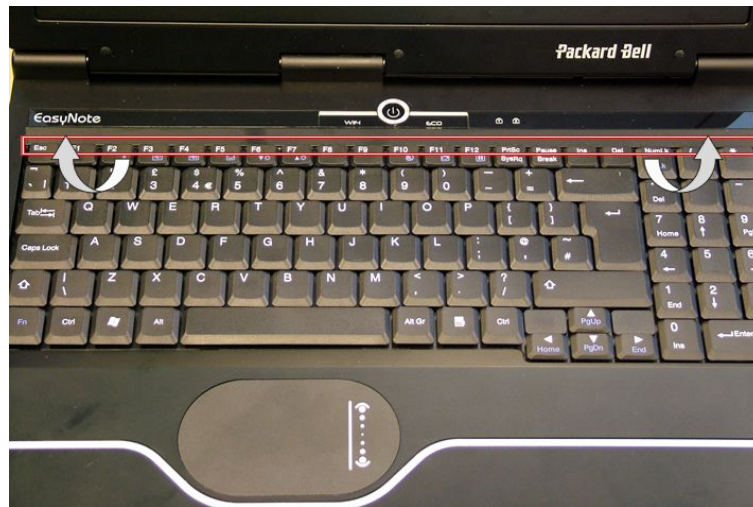
Fig. 11 Location of latches securing keyboard cover.
