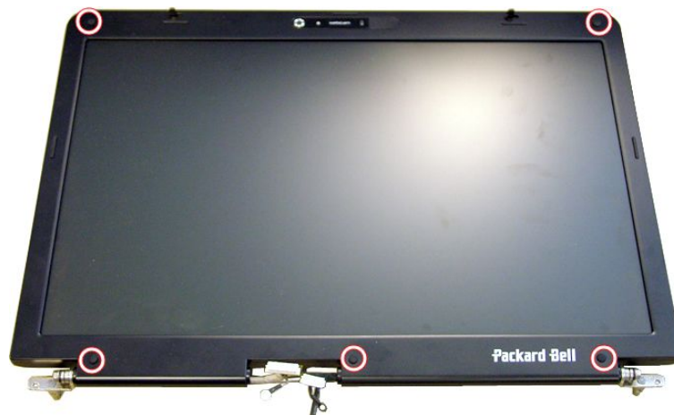
Fig. 26 Location of rubber stoppers.
