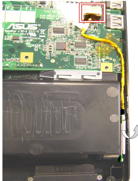
Fig. 21 Location of Bluetooth module and connector.
