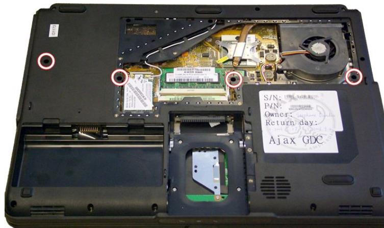
Fig. 10 Location of K> screws.
