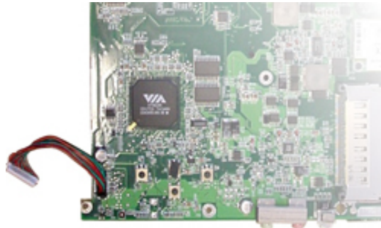
Fig. 33: Disconnecting the LED board assembly cable.
