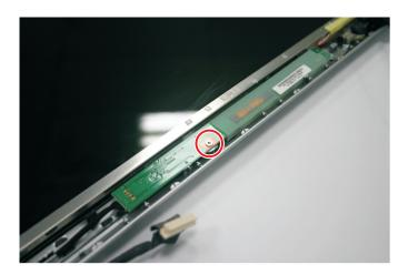
8 Turn over the inverter board to access the cables.
