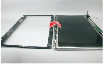
8 Remove the microphone from the LCD front panel.
