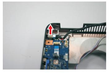
8 Replace the new dc-in cable into the base panel.
