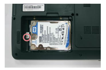
4 Grasp the black mylar tab and use it to disengage the hard drive from its connector, and then remove the drive from its bay.
