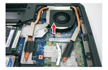
4 Loosen the spring-loaded captive screws securing thermal module. Follow the screw sequence indicated on the below images.
