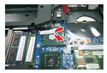
Remove the old processor from the system board.
