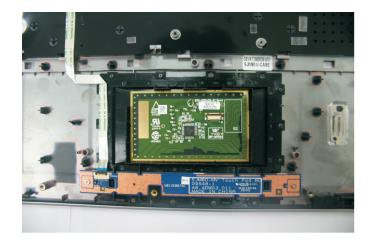
11 Insert a small flat-blade screwdriver or non-marring scribe between the touchpad board and the palm rest's underside, and carefully pry the board loose.
