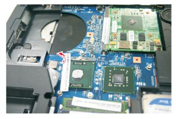
8 Moisten a soft cloth with isopropyl alcohol and clean the processor die to remove any thermal grease residue. Wipe the die surface several times to make sure that no particles or dust contaminants are evident. Allow the alcohol to evaporate before continuing.
