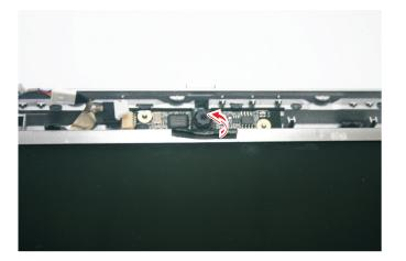
11~ Remove the LCD from the LCD assembly lid.
