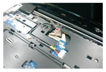
9 Disconnect the LCD and microphone cables from their system board connectors.
