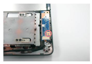
9 Release from latch and remove the USB board from the base enclosure.
