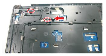
$11 \quad \mbox{Disconnect the left speaker cable from REAR2 connector and release it from the latch.}$
