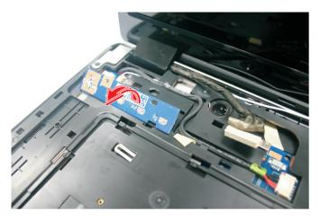
7 Disconnect the cable from the power button board and remove it from the system.
