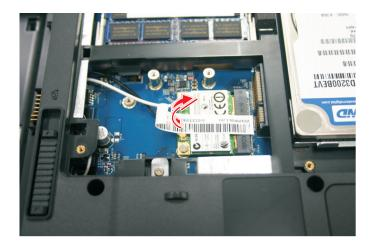
Unplug the antenna cables. Note which color cable corresponds to each of the connectors. 4
