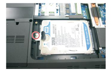
4 Grasp the black mylar tab and use it to disengage the hard drive from its connector, and then remove the drive from its bay.
