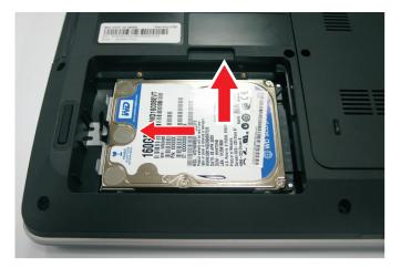
5 If your new hard drive already includes the hard drive bracket, go to step 9. If you need to use the bracket from the old hard drive, go to step 6. 6 Remove the screws that secure the hard drive bracket.
