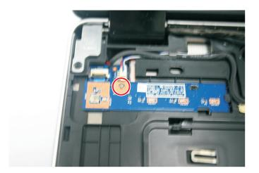
6 Carefully remove the power button board and turn in over to access the cable.
