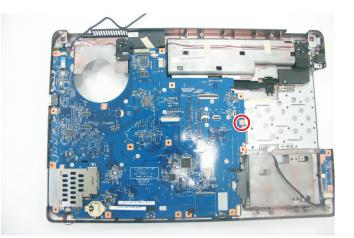
21 Remove the one screw securing the system board to the base panel.
