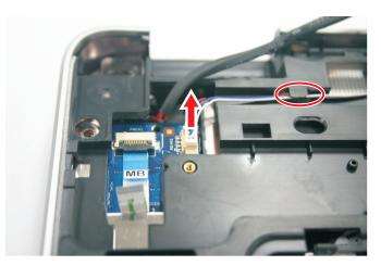
12 Disconnect the touchpad board and touchpad button board cables from TP335 and FP2 connectors.
