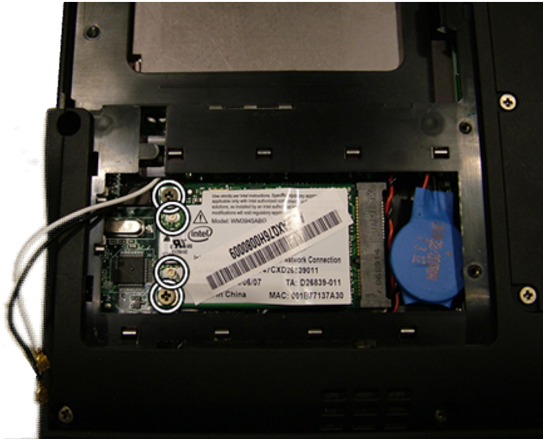
Fig. 6 The wireless LAN screws and cables.
