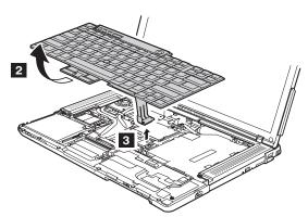
When installing: Make sure that the keyboard edges a are under the frame as shown in this figure.
