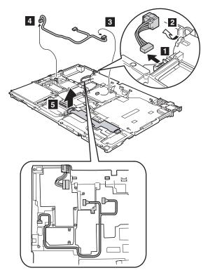
**When installing:** Make sure the connectors are attached firmly, and that the cables are routed as in the figure above.
