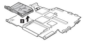
When installing: Make sure that the connector of PC Card/ExpressCard slots assembly is attached to the system board firmly.
