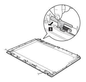
When installing: Attache the latches as shown in this figure.
