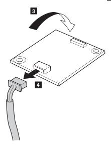
**When installing:** Make sure that the modem connector and the connector on the underside of the card are attached firmly.
