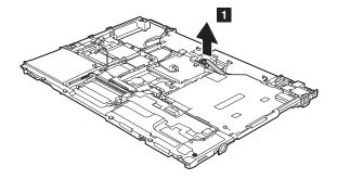
**When installing:** Make sure that the connector **1** is attached firmly.
