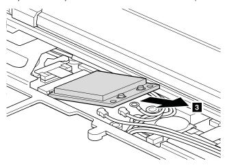
Note: Plug the red cable into the jack labeled MAIN on the card, and the blue cable into the jack labeled AUX.
