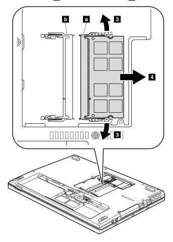
**When installing:** Insert the notched end of the DIMM into the socket. Press the DIMM firmly, and pivot it until it snaps into the place. Make sure that it is firmly fixed in the slot and does not move easily.
