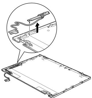
Table 35. Removal steps of LED sub card, LED cable, and LCD cover assembly (continued) Cable routing: When you install the LED sub card and LED cable, route the cable as shown in this figure.
