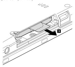
When installing: Make sure that the SSD connector is attached firmly.
