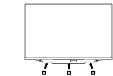
Table 31. Removal steps of LCD panel and LCD cable
