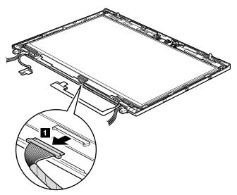
**Attention:** Unplug the LCD cable with holding the left and right edges of the connector with your fingers, and gently pull the connector toward you. DO NOT unplug it with pulling the cable. Applying tension could cause the cable to be damaged or a wire to be broken, and it might cause the S-driver to be damaged.
