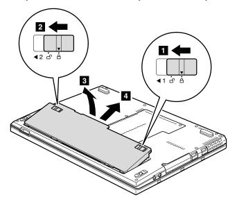
When installing: Install the battery pack along the slide rails of the slot. Then make sure that the battery release lever is in the locked position.
