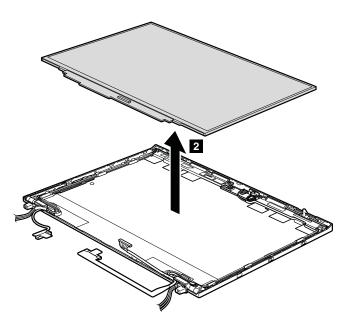
When installing: When attaching the LCD panel to the cover, press the left and right edges covered with metal gently with your fingers. DO NOT press the surface of the panel or apply any excessive force to the panel.
