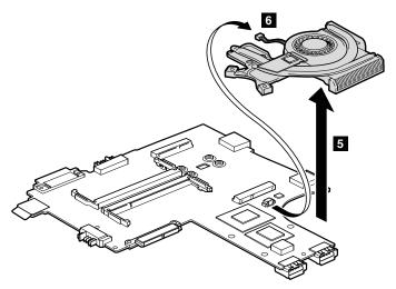
**When installing:** Make sure that the fan connector is attached to the system board firmly.
