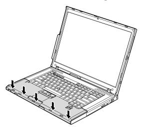
4. Close the LCD cover and turn the computer over. Then fasten the four screws in the order shown in this figure.
