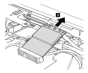
When installing: Plug the gray cable (MAIN) into the jack labeled TR1, the white cable (3rd) into jack labeled R0, and the black cable (AUX) into jack labeled TR2 on the card.
