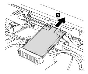
When installing: Plug the gray cable into the jack labeled MAIN on the card, and the black cable into the jack labeled AUX. If the computer you are servicing has three cables, put the white cable in the cable bag in the card slot.
