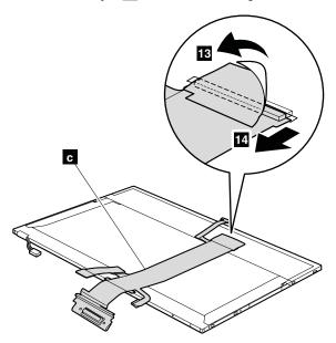
When installing: As you route the cables, make sure that they are not subjected to any tension. Tension could cause the cables to be damaged by the cable guides, or a wire to be broken.
