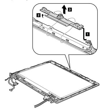
When installing: Make sure that the connector is attached firmly.
