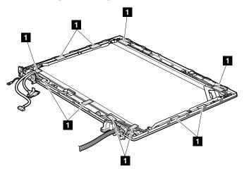
When installing: As you route the cables, make sure that they are not subjected to any tension. Tension could cause the cables to be damaged by the cable guides, or a wire to be broken.
