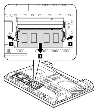
**Note:** If only one DIMM is used on the computer you are servicing, the card must be installed in SLOT-0 ( a : lower slot), but not in SLOT-1 ( b : upper slot).
