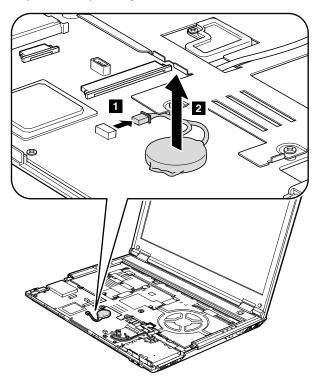
When installing: Make sure that the battery connector is attached firmly.
