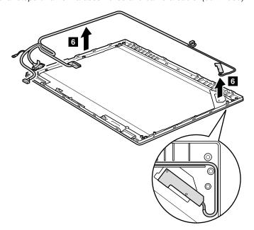
Table 40. Installation of the antenna assemblies and the camera cable
