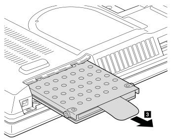
When installing: Make sure that the HDD connector is attached firmly.
