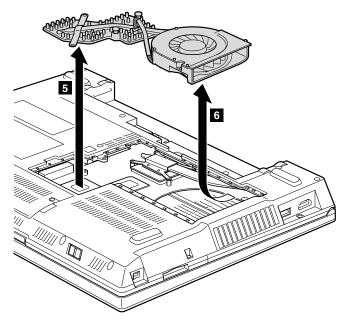
Table 20. Installation of the fan assembly
