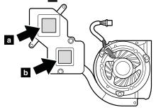
• Make sure that the fan connector is attached firmly.
