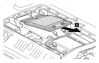
When installing: Plug the black cable with red label into the jack labeled MAIN, and the black cable with blue label into the jack labeled AUX on the card.
