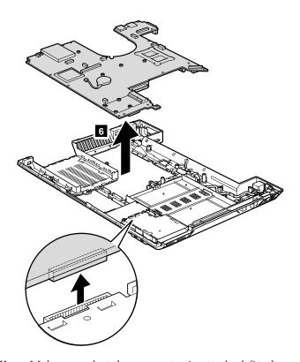
When installing: Make sure that the connector is attached firmly.
