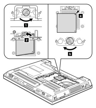
When installing: Place the CPU on the CPU socket a , and then rotate the head of the screw in the direction shown by arrow **b** to secure the CPU.
