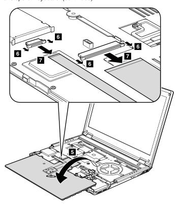
When installing: Make sure that the connectors are attached firmly.
