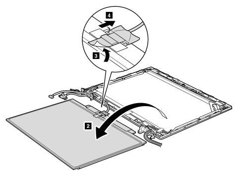
When installing: Make sure that the LCD cable is attached firmly.
