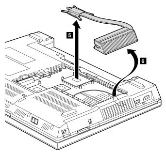
Table 22. Installation of the CPU thermal module
