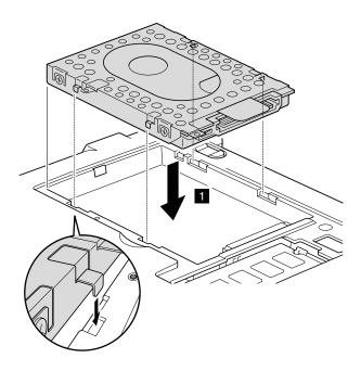
2. Slide the HDD in the direction of the arrow.
