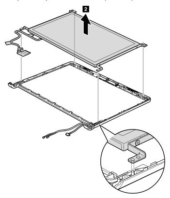
Remove the LCD brackets from the LCD panel.
