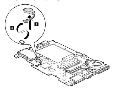
When installing: Make sure that the battery connector is attached firmly.
