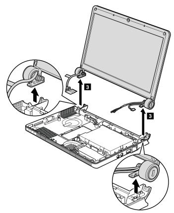
When installing: Route the LCD cable ( a ), the camera cable ( b ), and the wireless WAN antenna cables ( c ) along the cable guides. As you route the cables, make sure that they are not subjected to any tension. Tension could cause the cables to be damaged by the cable guides, or a wire to be broken.
