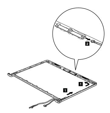
When installing: Make sure that the camera connector is attached firmly.
