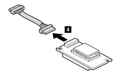
When installing: Make sure that the connector 4 is attached firmly.
