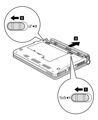
When installing: Install the battery pack along the slide rails of the slot. Then make sure that the battery release lever is in the locked position.
