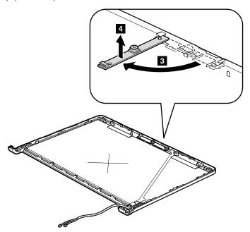
When installing: Route the camera cable as shown in this figure.
