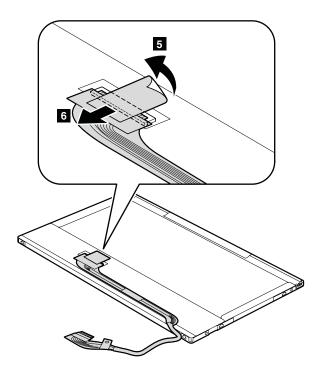
When installing: Make sure that the LCD cable connector is attached firmly.
