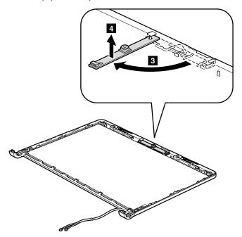
When installing: Route the camera cable as shown in this figure.
