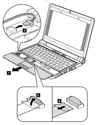
Turn the palm rest over, and then disconnect the cable from the flip-lock ZIF connector.
