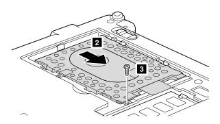
3. Close the HDD door, and then fasten the screws.
