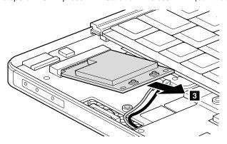
When installing: Plug the black cable into the jack labeled MAIN or 1 on the card, and the gray cable into the jack labeled AUX or 2.
