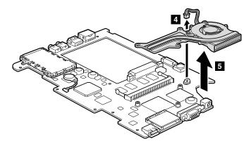
When installing: Make sure that the fan connector is attached to the system board firmly.
