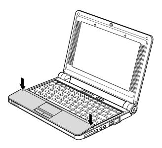
6. Close the LCD cover and turn the computer over. Then fasten the four screws to secure the palm rest.
