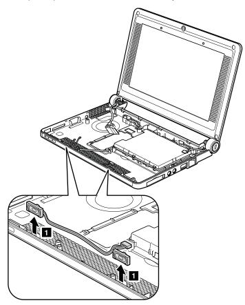
When installing: Route the speaker cables as shown in this figure.
