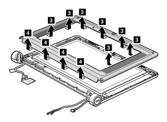
When installing: Make sure that all the claws are attached firmly.
