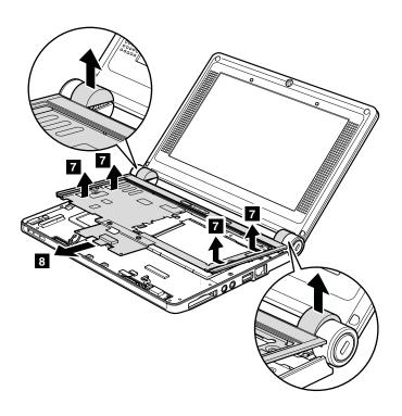
When installing: Make sure that all the claws are attached firmly.
