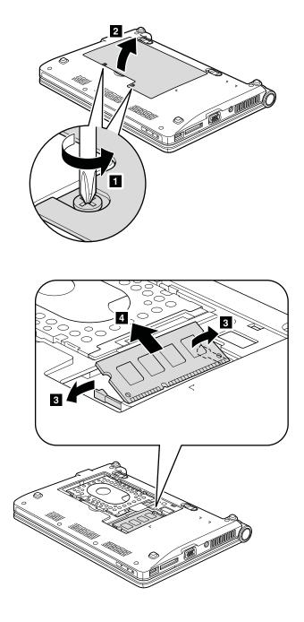
When installing: Insert the notched end of the DIMM into the socket. Press the DIMM firmly, and pivot it until it snaps into the place. Make sure that it is firmly fixed in the slot and does not move easily.
