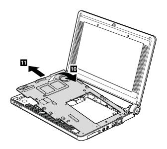
Note: The fan assembly is attached to the underside of the system board.
