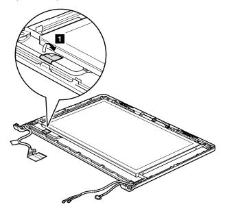
Table 31. Removal steps of LCD panel and LCD cable (continued)
