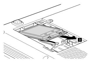
When installing: Plug the black cable into the jack labeled MAIN on the card, and the gray cable into the jack labeled AUX.
