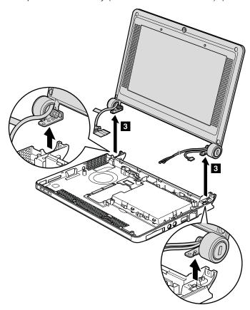
**When installing:** Route the LCD cable ( a ), the camera cable ( b ), and the wireless LAN antenna cables ( c ) along the cable guides. As you route the cables, make sure that they are not subjected to any tension. Tension could cause the cables to be damaged by the cable guides, or a wire to be broken.
