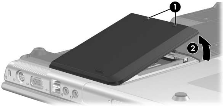
Removing the Hard Drive Cover
