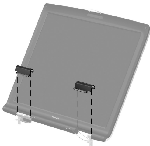
Figure 5-22. Removing the Display Hinge Covers
