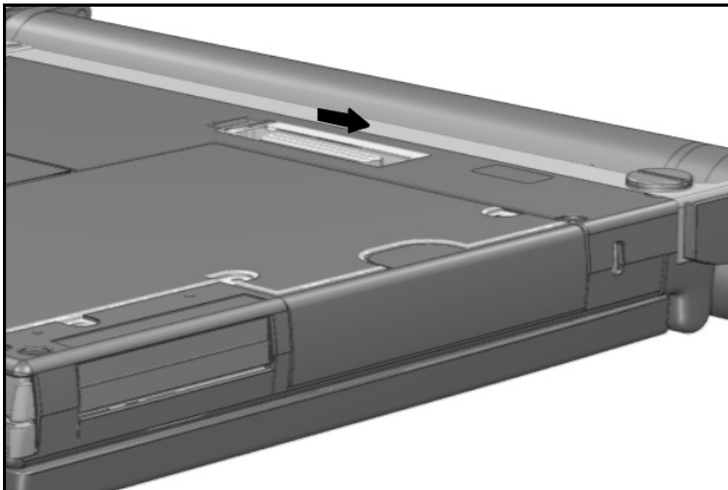
Figure 5-9. Closing the Expansion Slot Cover
