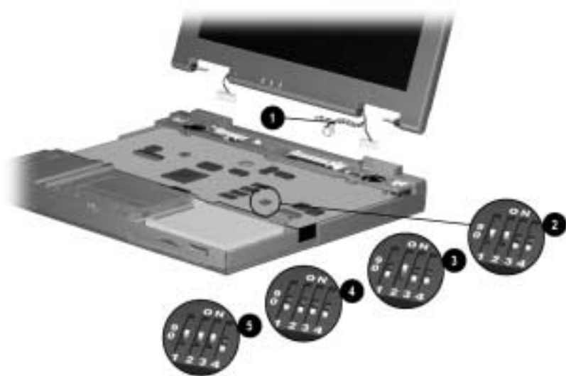
Figure 5-28. Setting the Display DIP Switches
