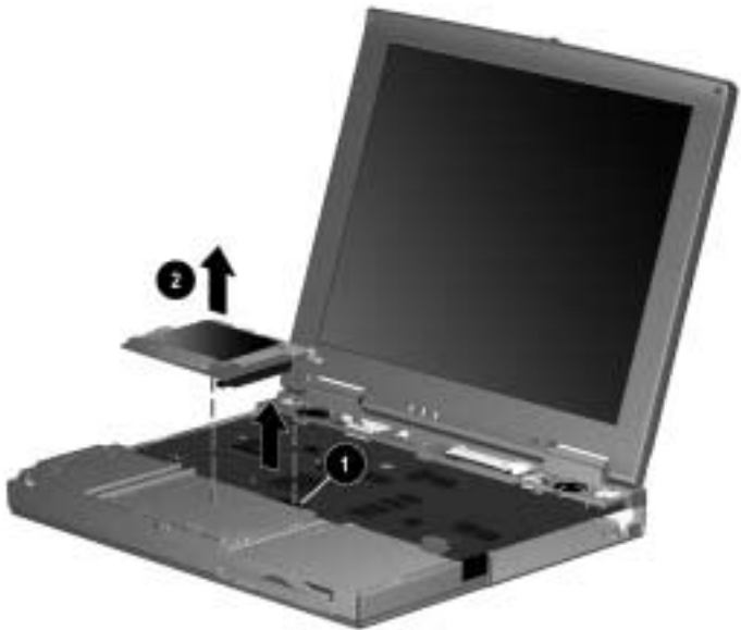
Figure 5-22. Removing the TouchPad
