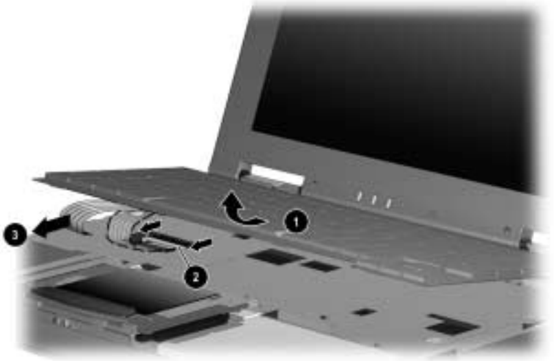
Figure 5-19. Releasing the Keyboard and Disconnecting the Keyboard Cable
