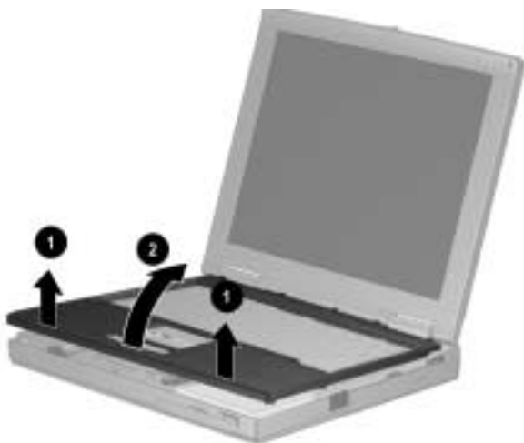
Figure 5-16. Removing the Top Cover
