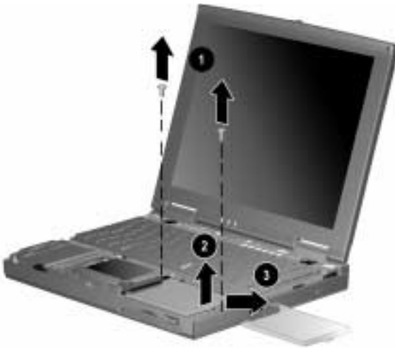
Figure 5-17. Removing the Hard Drive
