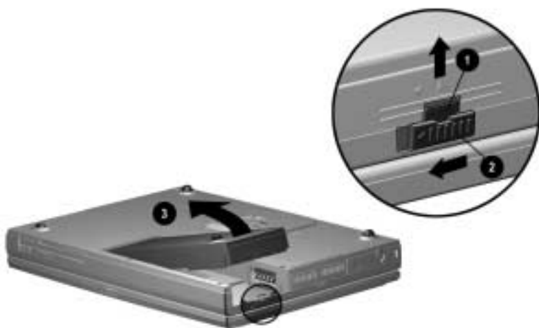
Figure 5-2. Removing the Battery Pack
