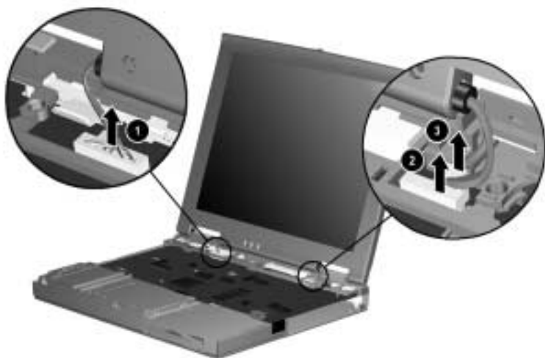
Figure 5-25. Disconnecting the Display Cables
