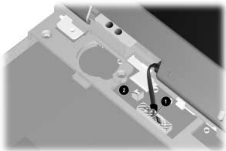
Figure 5-27. Routing the Display Video Cable
