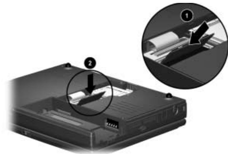
Figure 5-14. Installing a Memory Expansion Board
