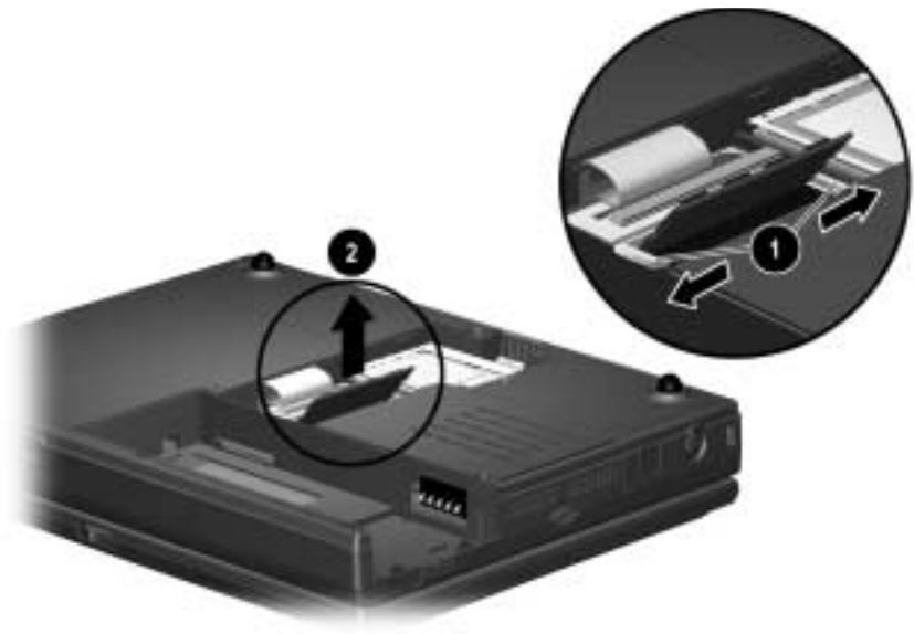
Figure 5-13. Removing a Memory Expansion Board
