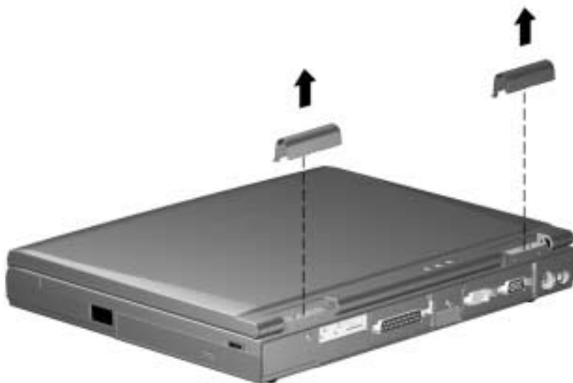
Figure 5-24. Removing the Hinge Covers
