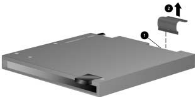
Figure 5-35. Disconnecting the Diskette Drive Cable
