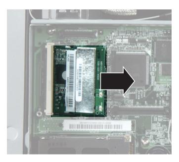
**8** Insert the new Mini PCI card into the slot, then press it down until the retaining clips snap into place. The card must be fully seated in the slot before the retaining clips will snap into place.
