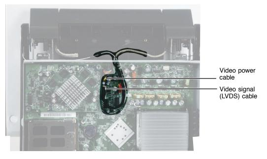
**5** Disconnect the video signal (LVDS) cable and video power cable from the system board.
