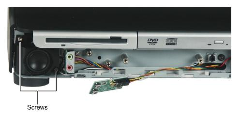
**8** Remove the two screws from the speaker you are replacing.
