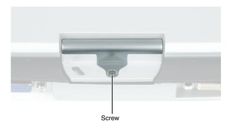
Insert the small flat-blade screwdriver or non-marring tool under the bottom of the hinge cover, then carefully pry it up.
