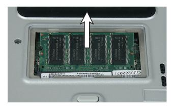
**6** Pull the memory module out of the slot.
