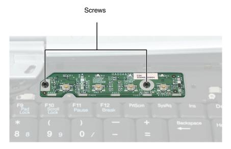
**8** Insert the small flat-blade screwdriver or non-marring tool under the edge of the LED panel, then carefully pry it up.
