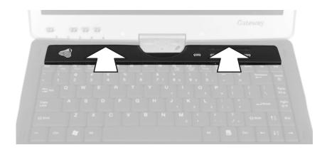
10 Press down on the keyboard cover in several places to make sure that it is correctly mounted. The keyboard cover is correctly mounted when you can run the finger along the keyboard cover and find no loose spots. The keyboard cover should be flat all the way across.
