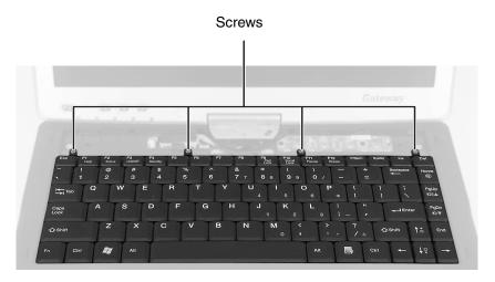
**17** Replace the keyboard cover and battery, connect the AC adapter and modem and network cables, then turn on the convertible tablet PC.
