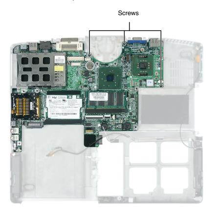
**26** Remove the system board. Make sure that the rear I/O panel clears the bottom of the chassis and the side audio jacks clear the bottom of the chassis.
