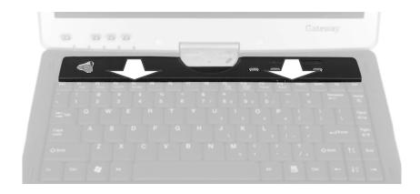
**9** Slide the tabs on the bottom side of the new keyboard cover under the convertible tablet PC frame.
