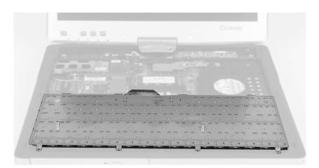
**8** Carefully insert the small flat-blade screwdriver between the keyboard cable and the black plastic hinge where the cable connects to the system board. Gently lift the hinge off the cable. The cable is now free and you can remove the keyboard.
