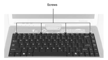
**7** Lift the back edge of the keyboard, then slowly rotate it toward you so it lies **keys-down** on top of the convertible tablet PC. Be careful not to damage the LCD panel.
