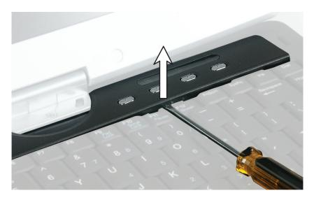
**8** Remove the keyboard cover from the convertible tablet PC by pulling the keyboard cover toward you and at the same time lifting its front to clear the keyboard. You will hear small snapping sounds as the keyboard cover comes away from the convertible tablet PC. Be careful not to break off the tabs found on the bottom of the keyboard cover.
