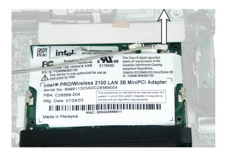
17 Move the antenna wires out of the way, then press outward on the clips at both sides of the card until the card tilts upward.
