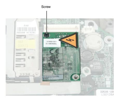
**14** Insert the small flat-blade screwdriver or non-marring tool under the modem and gently pry it up about ¼ inch.
