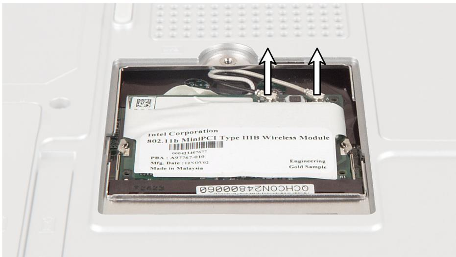
*Replacing the IEEE 802.11 Mini PCI card*
