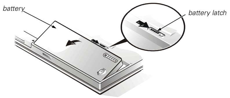
Figure 2. Main Battery Assembly Removal
