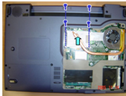
Figure 2-5 Free the heatsink
