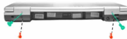
Figure 2-19 Remove four screws
