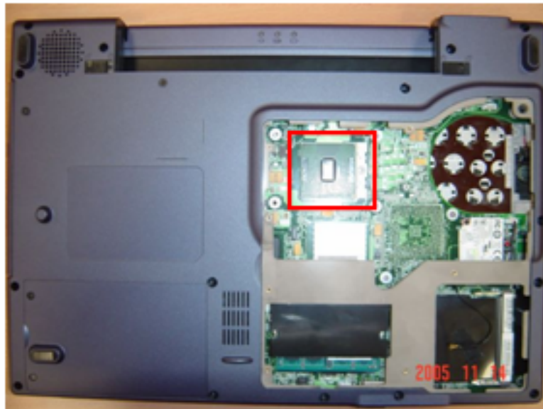
Figure 2-6 Remove the CPU
