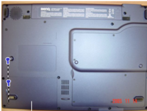
Figure 2-7 Remove the HDD cover
