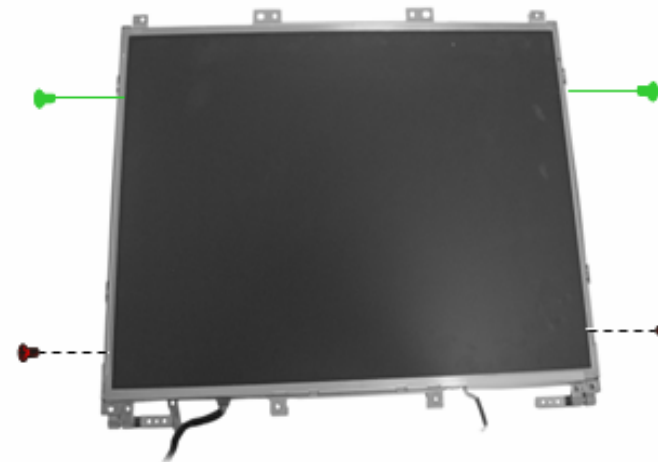
Figure 2-27 Remove 4 screws to release LCD Hinge bracket
