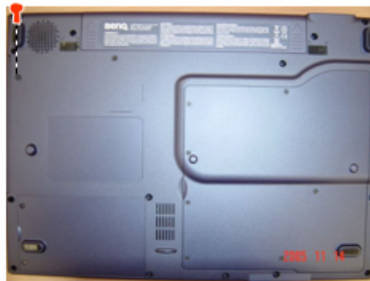
Figure 2-10 Remove one screw
