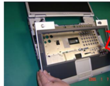
Figure 2-20 Free the Top Case
