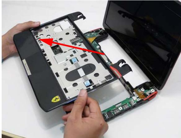
14. Remove the I/O board to main board cable.
