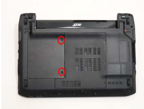
3. Remove the HDD Cover from the inside edge.
