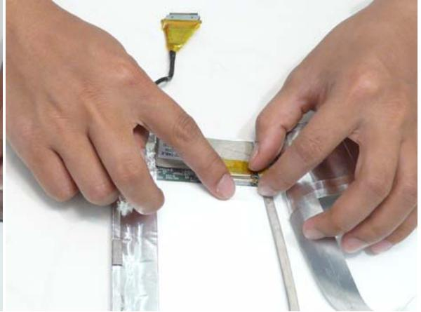
5. Apply adhesive and press down the FPC cable sleeve.
