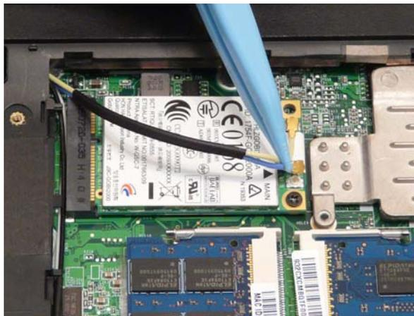
5. Remove the one (1) screw from the 3G module.
