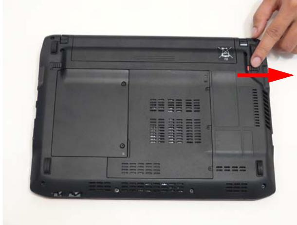
3. Slide and hold the battery release latch to the release position (1), then slide out the battery pack from the main unit (2).
