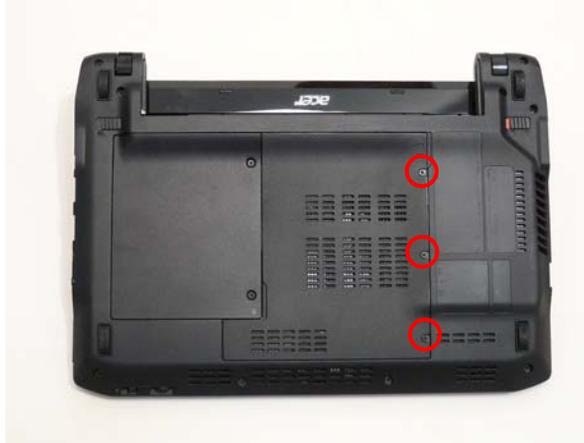
3. Replace the HDD cover, aligning the outside edge tabs first.
