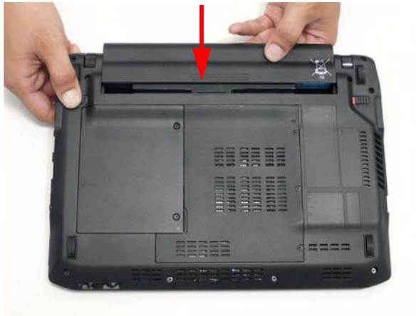
2. Slide the battery lock switch into the closed position.
