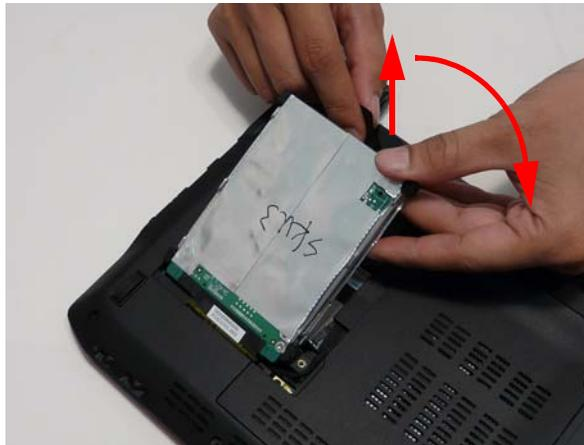
6. Grasp the HDD cable connector tab and pull up.
