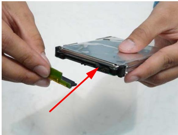
3. Connect the HDD cable to the main board.
