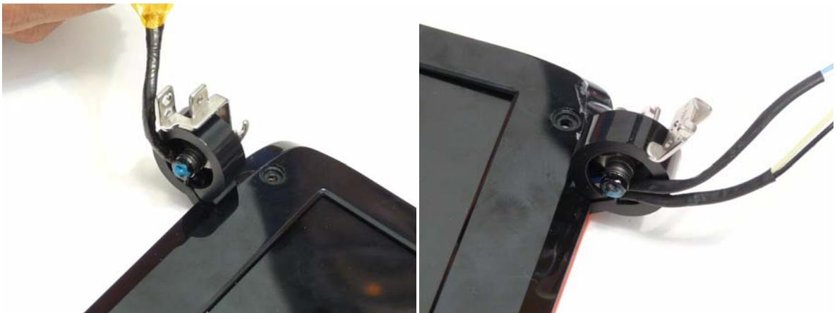
2. Press the bezel down around the edges.
